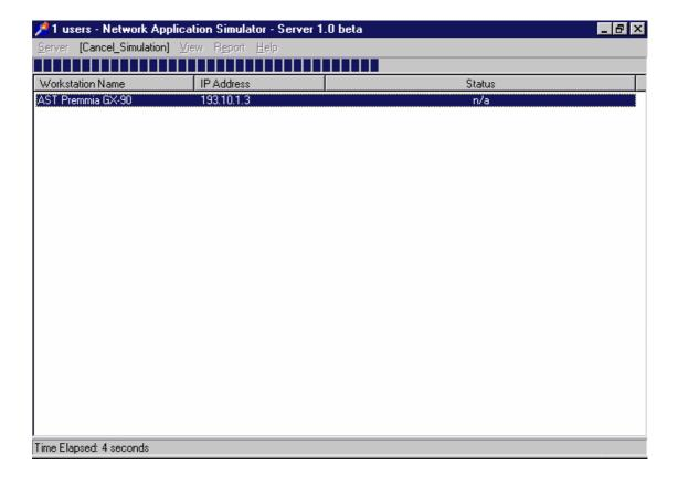
After we set all options properly, we may start the simulation by selecting any client and clicking on the "Run" menu. All menu items will be disabled, and "Run" menu will be changed into "[Cancel\_Simulation]". By selecting that menu item, the user can cancel the simulation at any time. A sample of the software in action is available from the screenshot above.
