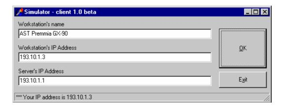
When the user press OK, the software will try to establish connection to the server. If it failed, it will inform it to the user. If it succeed, it will register itself to the server, and start the auto-reconnect feature.
